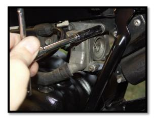
7) Remove the two 10mm bolts which hold the SAI unit to the frame and lift the unit clear of the bike.
