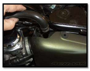
4) Pull away the large rubber hose that sucks air from the air box and seal the hole with the supplied plastic bung.
