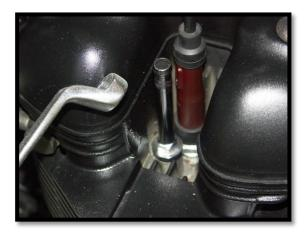
8) Use a 13mm ring spanner remove both the chrome tubes, apply some copper grease to the threads of the alloy bung, place a copper washer on the bung and with a 6mm hex key/socket torque to 12Nm. Repeat for the other side.
