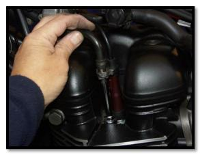
3) Disconnect the black tubes connected to the chromed tubes screwed in to the cylinder head by the spark plugs by wheedling them gently with upward pressure to pull them off.
