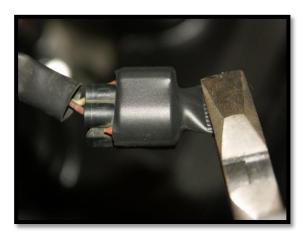
5) **EFI MODELS**: Unplug the electrical connector from the SAI unit and place the supplied heat shrink over the remaining loom electrical connector and use a heat gun to shrink to size. With the heat shrink still hot, clamp the open end with a pair of pliers to seal from the elements. **Do not** use your fingers, the heat shrink is far too hot.
