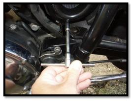
5) Replace the three OEM 8mm bolts in the Breathe cover and tighten to 3 Nm.
