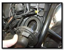
4) Replace the OEM cover/snorkel with the Breathe cover and don't forget to swap the large sealing O ring from the OEM cover to the Breathe.
