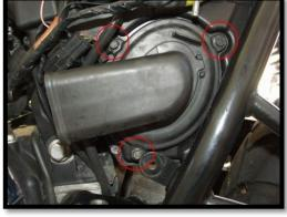
3) Remove the three 8mm bolts from OEM cover/snorkel.
