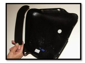
6) If you frequently ride in wet weather, then it's a good idea to fit the splash strip provided to the rear of the side panel. Clean the side panel where you will stick the strip and remove the backing paper on the splash strip stickies.
