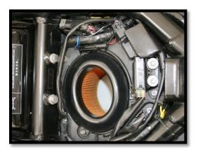
Install the Breathe in place of the OEM snorkel/intake cover and replace the three 8mm bolts and tighten to 3 Nm. Then replace the wiring cover and seat.
